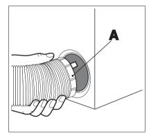
If the hose is long and the room temperature low, the moisture might condense to water inside the hose. This is an unavoidable natural phenomenon. To prevent this water from lying in the hose or flowing back into the tumble dryer, it is advisable to drill a small hole (via. 3 mm) in the lowest point of the hose and to place a small container below it. (See picture, point B).
